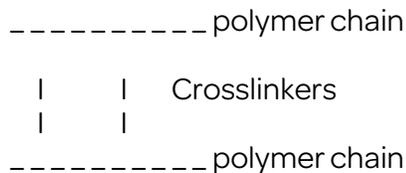
The crosslinkers make movement more difficult. This is similar to adding borax to the glue solution. The chain here gets more inflexible as the glue got thicker.
